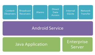
Fig. 1. DroidWatch system architecture.
