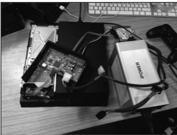
Fig. 3. Tableau T32is used as a man-in-the-middle between the PlayStation 4 and its hard drive.
