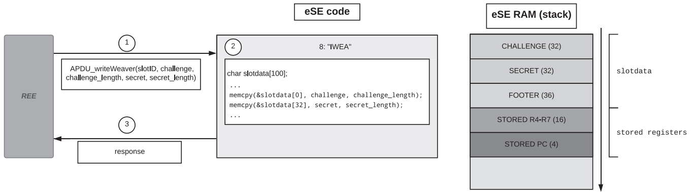
Fig. 3. Buffer overflow in eSE APDU_writeWeaver handler.
