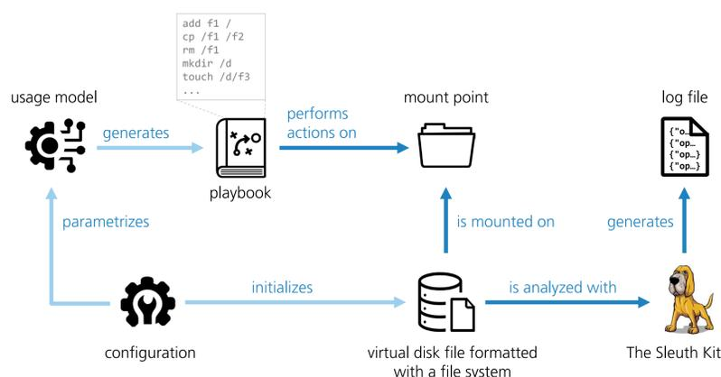
fsstratify uses playbooks to define operations, such as creating, modifying, or deleting files, to be performed on a mounted file system. The execution is carried out by the host operating system using its file system implementation. Playbooks can be written manually using a simple syntax or they can be automatically generated based on usage models implementing a certain use of the system (e.g. office usage, web server etc.).
