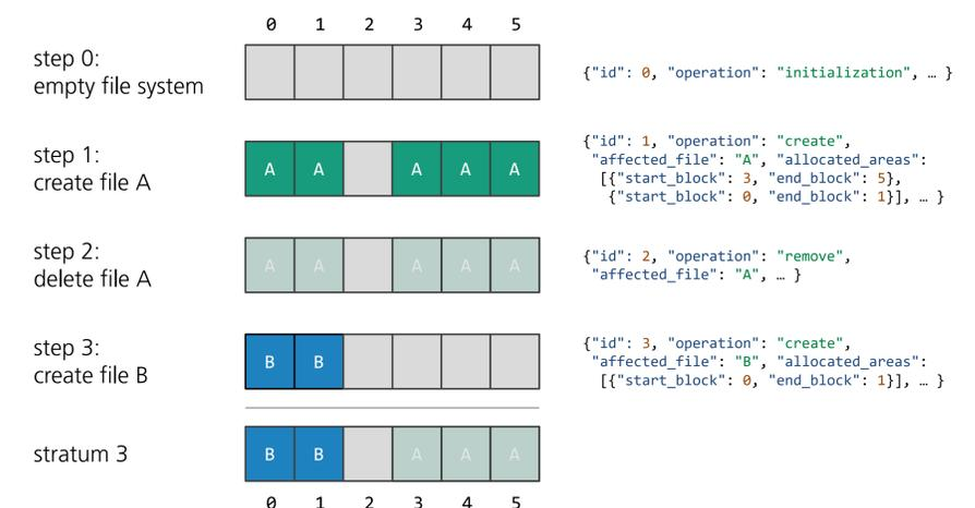
Analyzing file system strata opens up various possibilities. It enables detailed studies of file system implementation behavior and we can easily conduct large-scale experiments regarding fragmentation or allocation strategies for both, different file systems and different operating systems. Moreover, we can use fsstratify to create disk images for testing data recovery techniques. The strata provide an accurate ground truth about what is still recoverable and what has already been overwritten.
