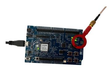
**Fig. 3.** Acquisition of electromagnetic (EM) traces while carrying out various software activities on the Nordic Semiconductor nRF52-DK using the HackRF One SDR connected with h-loop near-field antenna.
