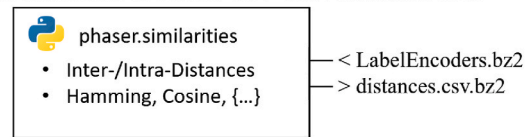
(b) Calculate inter- and intra-distance scores. Intra-scores comparisons are 1:1 original to transformed, while inter-scores are sampled to match the total number of intra-distance observations. Distance metric labels are also encoded.
