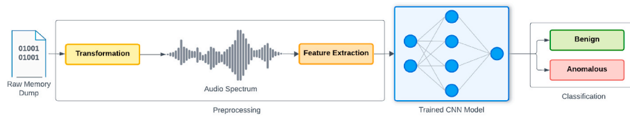
Fig. 4. Overview of memory-based anomaly detection algorithm.
