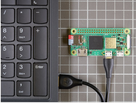
Figure 2: Setup of USB device emulation with Raspberry Pi Zero 2 W
